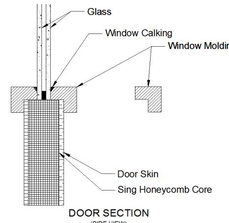
The standard 1 1/2" solid wood edging is adequate for door hinges but add solid wood blocking to your door core for added hardware or door knob needs.
